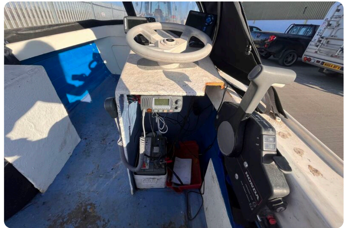
Fisherman 17 clinker boat - steering wheel and engine controls
