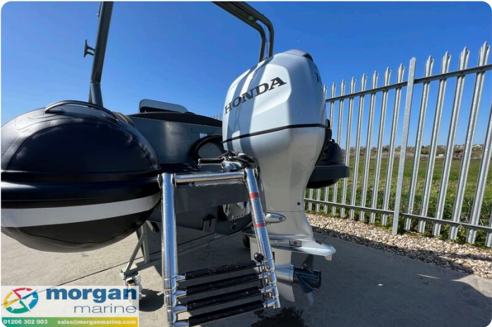
Highfield Sport 520 aluminium RIB - Honda BF100 outboard engine
